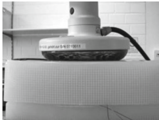
Fig. 7: Agar-muscle phantom: AGAR 4% + NaN3 0.9% dim. 18 x 30 x 35 cm 3
